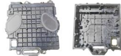
Housing of HV inverter for EV High pressure Die casting, FSW, critical tightness & cleanliness
